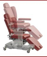
**Variable height adjustment** via motorized telescopic column with rectangular section with a <u>capacity of 200 kg and an excursion of 400 mm.</u>
