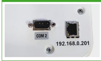
Activation of the interface Ethernet/LAN port on Fly Plus model balance display.
