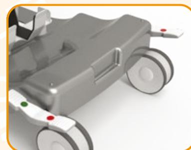
FREIN CENTRALISÉ AVEC SYSTÈME DIRECTIONNEL
