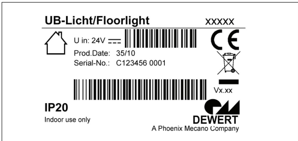
Figure 1 Rating plate example
