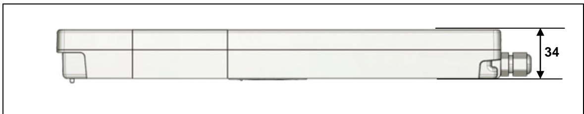
Figure 5 Dimensions of the AG300, side view (in mm)
