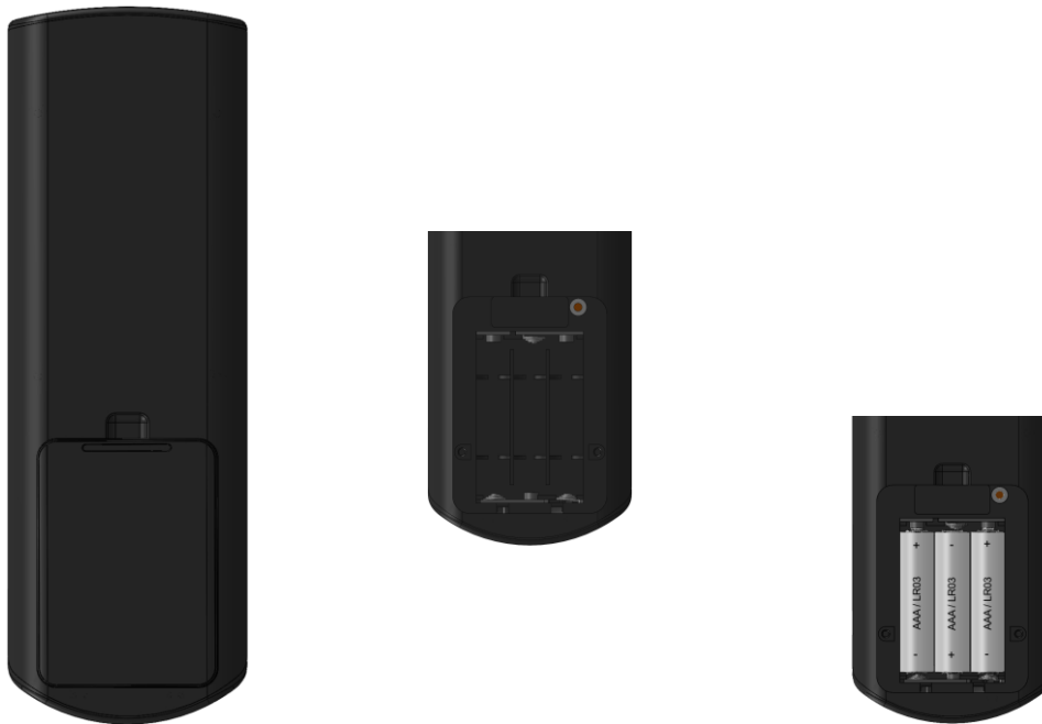
Figure 6: Changing the battery in the RF-TOUCH hand-held remote control
